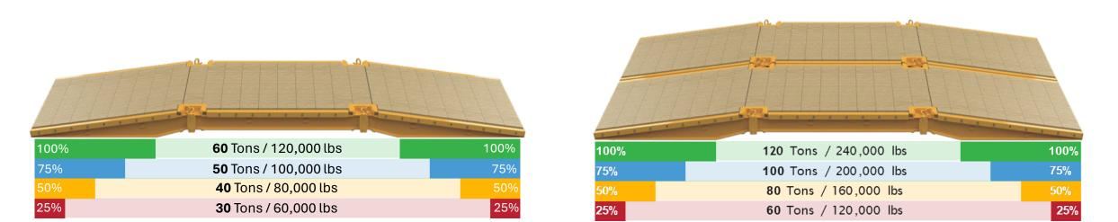
Load ratings based on stable foundation - ratings may vary, dependent on soil or foundation conditions. Site review and inspection are recommended to ensure a stable foundation.
